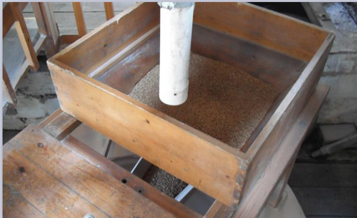
The hopper for holding wheat
